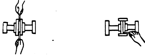
Figure 3B. Aligning Non-Spider Type Couplings
